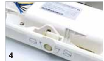
4 The enclosure and transparent shield are pressed tightly and drive the switching off and interlocking function of explosion-proof distance switch by unlocking device through interlock mechanism.
