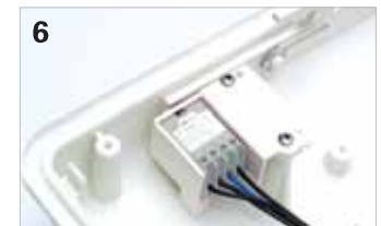
6 The explosion-proof distance switch module of Ex de IIC is operated by interlocking device and the enclosure can only be opened when the switch is off.
