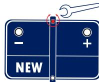
Clean corroded parts in tray and cable clamps, before installation of new battery.
