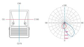
note : photometric result tested based on 11000lm MH 150W double ended tube
