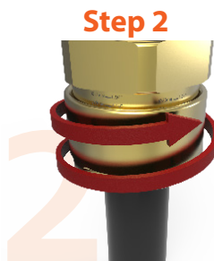
Tighten backnut until a seal is formed onto the cable, then tighten one further turn
