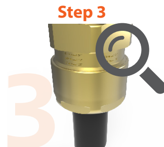
The backnut should be level with the marking guide corresponding to its diameter – this can be visually inspected and adjusted as necessary
