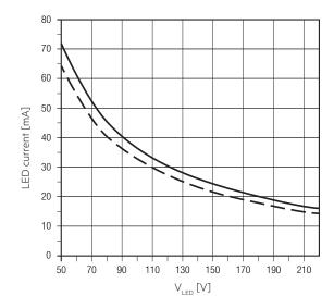
LED current at nominal battery voltage and min. battery discharge current
