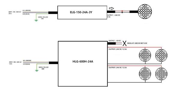
(Our crane light works on 9-60V DC, if you have this available on your cranes you can wire the lights directly to it. If you have only AC power, then you will need an AC-DC converter. We recommend you model ELG-150-24a from www.meanwell.com)
